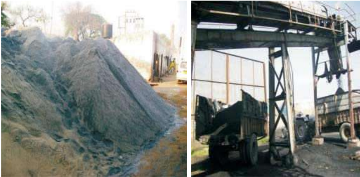
Fig 5.13-Fugitive Emissions from Boiler Ash temporary storage area
