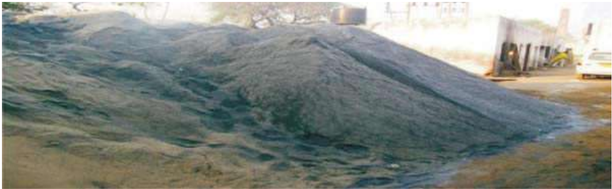
Fig 4.14-Open storage of husk fired boiler ash
