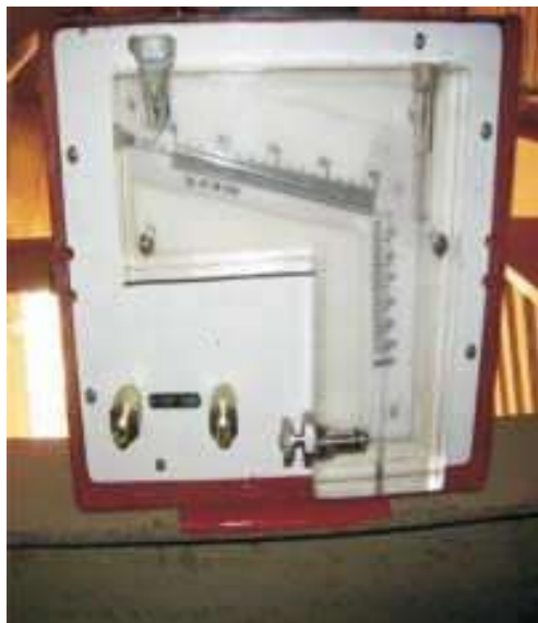
Fig. 6.1 Inclined Manometer used for Velocity Measurement
