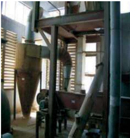
Fig. 4.4- Dust extracted through Cyclone
