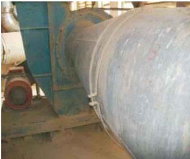
Fig 5.21-Suction ducts from polisher to cyclone for bran separation in small rice mills
