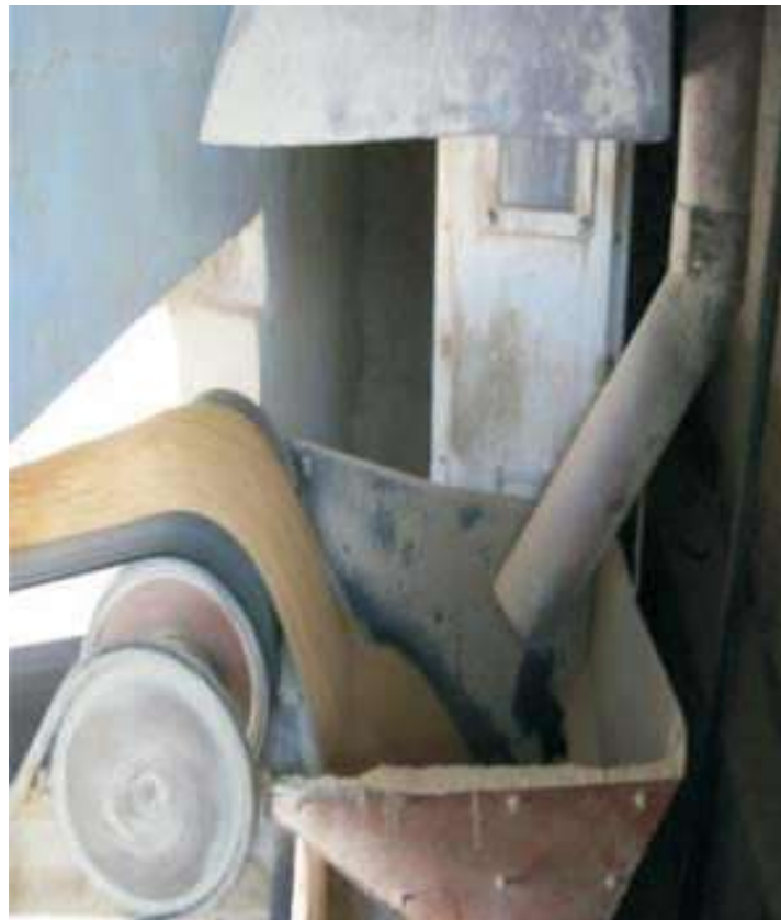
Fig 5.16-Extraction Hood near Bucket Elevator in large mills
