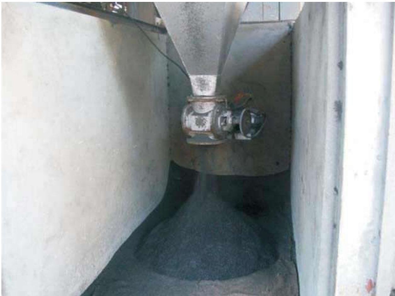
Fig 5.22- Cyclone for collection of boiler ash in large and medium rice mills
